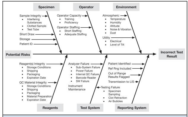
**Fig. 3.** Quantra System fishbone diagram for the identification of potential errors and mitigations, adapted from the CLSI EP23-A Workbook (3). ID, identifier; LIS, laboratory information system; SW, software.
