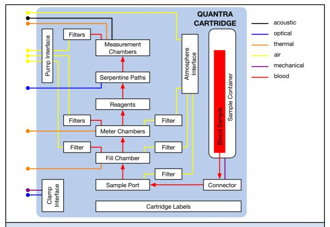
**Fig. 1.** Schematic representation of the single-use cartridge used with the Quantra Hemostasis Analyzer. The key functional pathways of the cartridge are highlighted in different colors. The combination of various interfaces between the cartridge and the analyzer enables the implementation of the internal QC checks described in this article.
